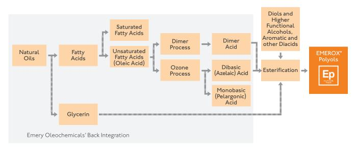
Process flow chart of EMEROX<sup>®</sup> polyols. Gray box demonstrates Emery Oleochemicals' long history and consistency with this process, including our back integration and unique process technology. The esterification process allows for the design freedom to customize value-added solutions for our customers and partners while combining the benefits of our long history, consistency and quality.
